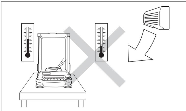
**Install the balance away from heating and air conditioning air current.**
