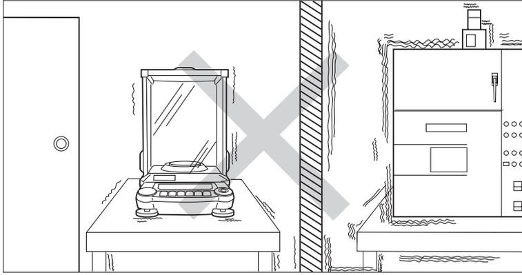
**Install the balance where it is free of vibration.** Any vibration transmitted from machinery or traffic may reduce the stability of measurements.
