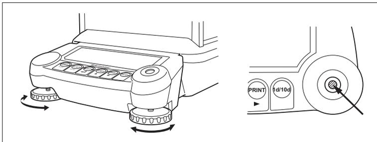
**Perform level adjustment.** Correct measurement cannot be performed if the balance is not leveled.
