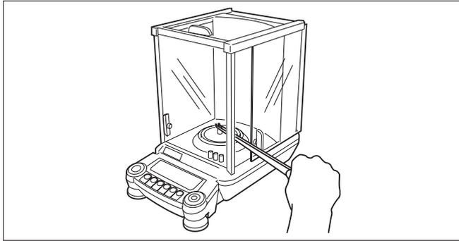
**Especially in the semi-micro range measurements, use a long pair of tweezers as much as possible.** Inserting the hand in the balance chamber generates air convection as human body emits heat. Convection may make measurements unstable.
