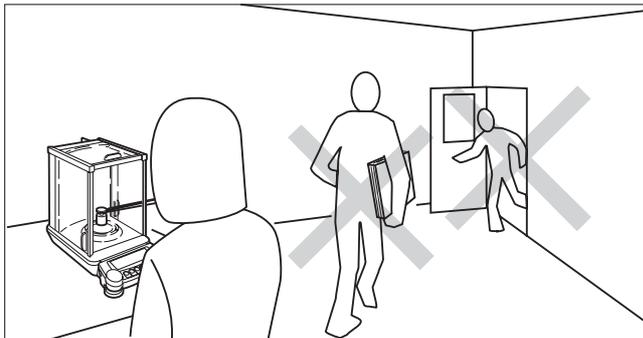
**Especially with the semi-micro range, avoid the movement of people into or around the room during measurements.**
